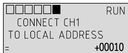
Fig. 3.1 – Selecting the monitor that channel 1 will control
