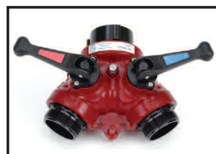
A wye with folding handles and a unique half-ball gate, introduced by Task Force Tips, reduces friction loss in the appliance and prevents the gate from opening wide during high-pressure water flows. (TFT Photos)
