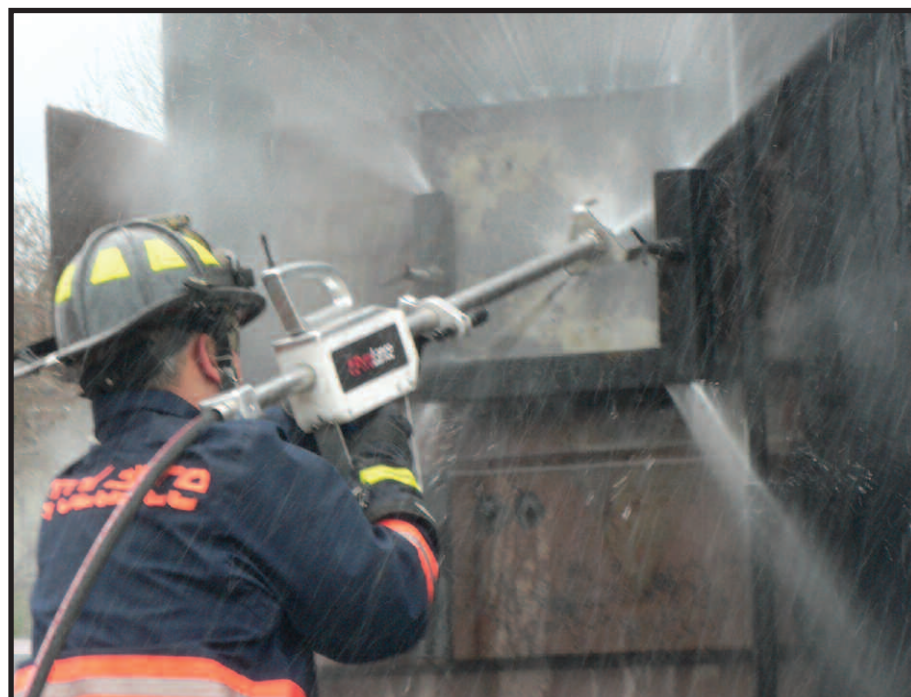
The makers of PyroLance, a high-pressure piercing nozzle system, demonstrated their product at FDIC. The system uses water and cutting aggregate discharged at 4,500 psi to pierce materials to administer atomized water to cool fires. (Fire Apparatus Photos by Ed Ballam)
